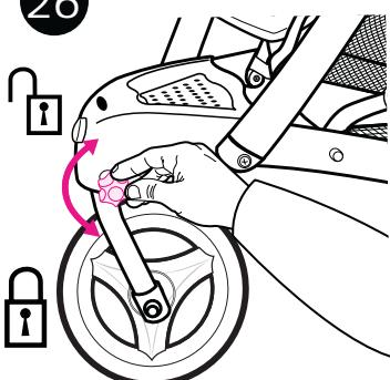
Front swivel wheel locks for use on uneven surfaces such as grass, stones or gravel.
